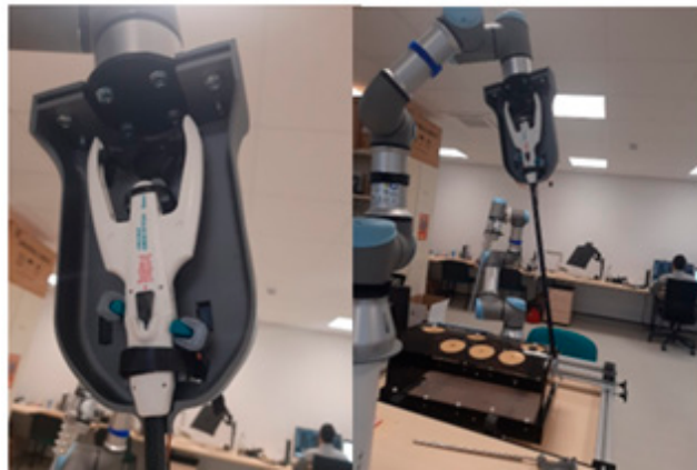
Figure 16. Device with the Endo Stitch gripper attached to the UR3 robot. Source: own.
